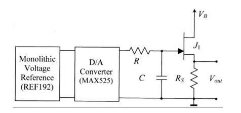
• In low frequency noise applications electrolitic capacitors cannot be used due to micro discharge effects that translate into high low frequency noise contributions.
