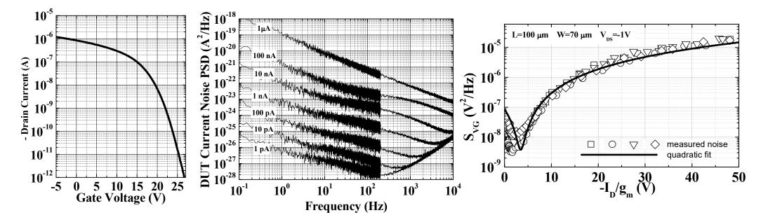
> 1/f noise measured down to 1pA; the sample size (number of measurement in different bias point and devices) is unprecedented for this type of investigation.
