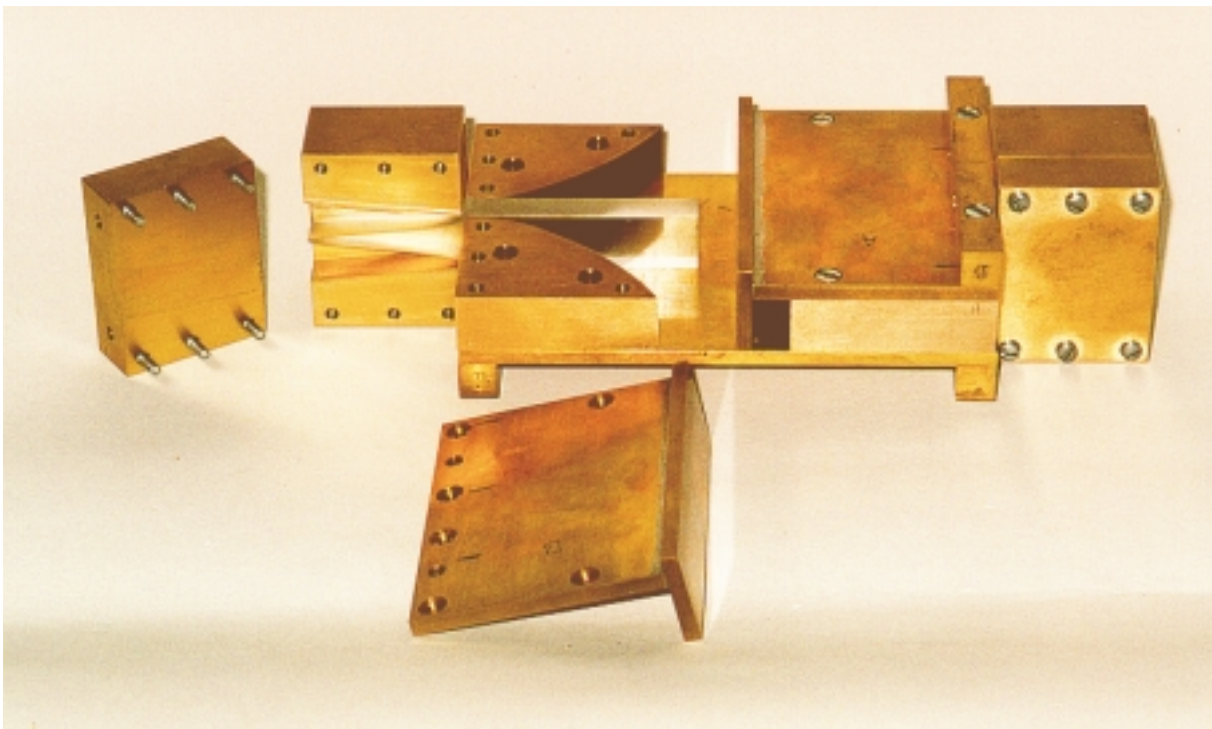
Figure B.3: The "reflect" calibration circuit of the X-band NRD-guide calibration kit. The closing metal plates are taken away to demonstrate the entire circuit.
