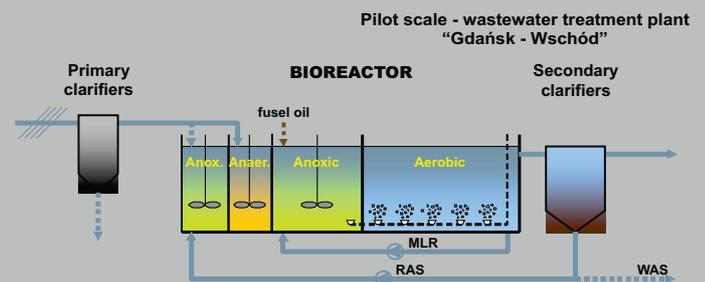
Fig.2. Scheme of pilot scale JHB system.
