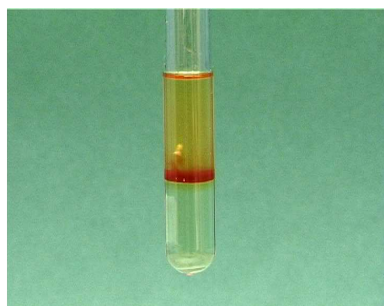
Fig. 2a. The correct course of the reaction leading to nitrobenzene as its product.
